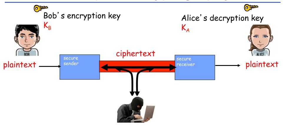
symmetric key crypto: identical sender and receiver keys public-key crypto: encryption key *public*, decryption key *private*
