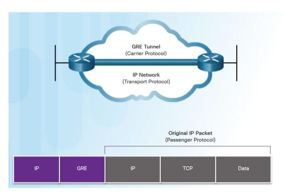
A tunnel interface supports a header for each of the following:
