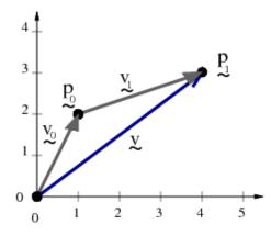
Here we see we are adding the vectors  $\mathbf{v_0}$  and  $\mathbf{v_1}$  to get a new vector  $\mathbf{v}$ , where:
