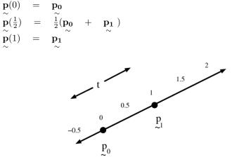
So, we can imagine that at "time" t = 0 we are at the point  $\mathbf{p_0}$ , and as "time" increases we move along the line so that when t = 1 we are at the point  $\mathbf{p_1}$ . As t keeps increasing, we travel along line and we talk about the number of *steps* we have taken from  $\mathbf{p_0}$ , for example when t = 2, we have taken 2 steps along the line.
