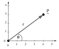
For the point shown, the distance from the origin to the point, r, is 5, and the angle  $\theta$  is 36.8699° (or 0.6435 radians, since we use radians to measure angles - remember, a full circle has 360°, and  $2\pi$  rad).
