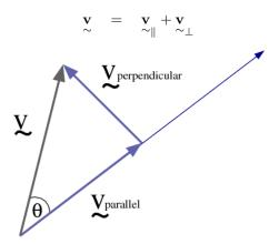
If we recall the results for a right angled triangle, then  $|\mathbf{v}_{ij}| = |\mathbf{v}| \cos(\theta) \ldots$ which means we can use the dot product of the two vectors to get the component of the vector that is parallel. As a result, we do not have to explicitly calculate the angle,  $\theta$ .
