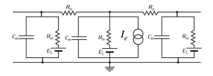
• For the compartment j, the total electric current is the sum of the capacitive current, leftward and rightward axial currents and in general also external current (from electrode or synapses). Thus:
