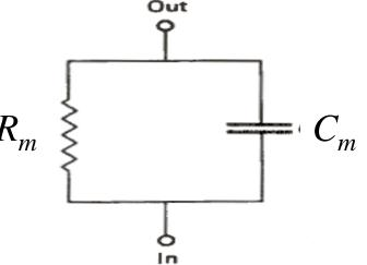
This is called an RC circuit in electronics since it consist of a resistor and capacitor.
