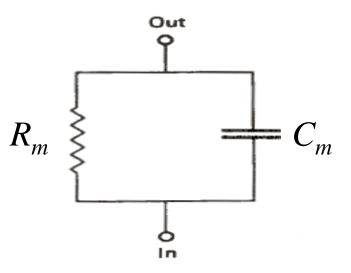
By convention capacitance current is 'plus' while membrane current is 'minus':
