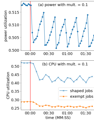
Figure 6: Power and CPU utilization during a load shaping event with multiplier 0.1 that directly affects a subset of tasks. The red vertical line marks the start of the event. The CPU reduction of the load-shaped tasks are more prominent than that of the exempt tasks. The exempt tasks are indirectly affected because of their interaction with the shaped tasks. (The power and CPU readings are not exactly time-aligned due to sampling delays.)
