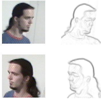
Figure 35 Edge strength results. The left images are the original; the right images represent the edge strength. The darker pixels represent the stronger edges.
