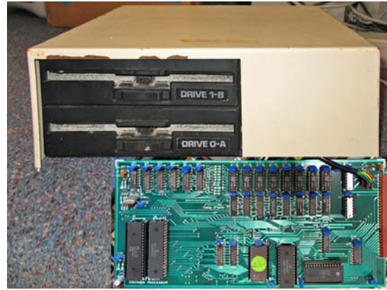
(b) A Proteus server and its CPU and memory board (inset)
