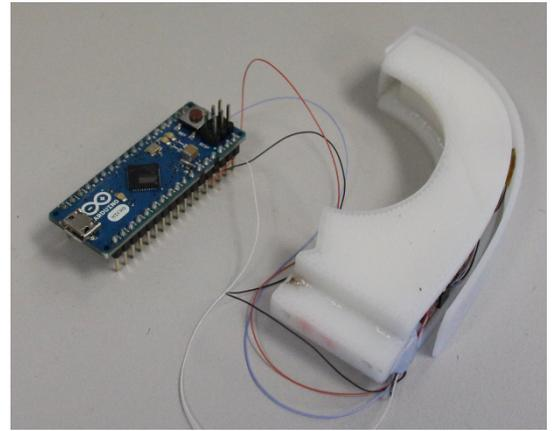
Fig. 3. The printed arm of the gripper with sensors and controller and outer skin
