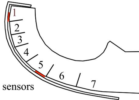
Fig. 5. Diagram of the gripper showing sensor placement
