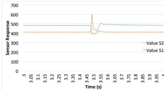
Fig. 10. Sensor response to an impulse force at Sensor 2
