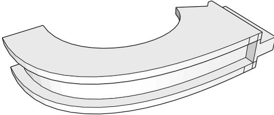
Fig. 1. Design model for one arm of the gripper design
