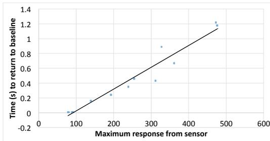
Fig. 9. Time for the sensor to recover versus the initial sensor response
