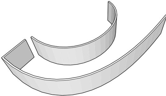
Fig. 2. Design model for outer skin of the 3D printed gripper
