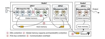
Figure 1: An example of deploying GPU microservices.
