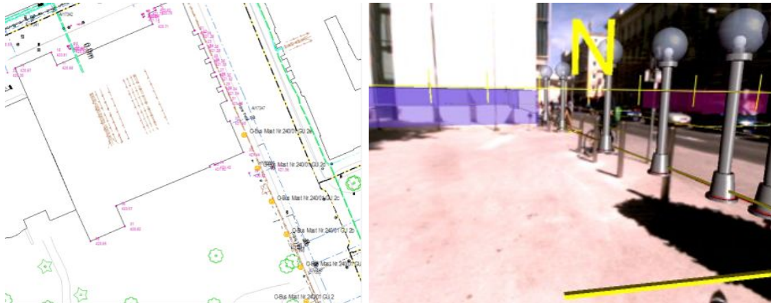
Figure 2.21: Traditional paper plans vs. an AR interface for planning. Left) Paper-based planning, newly planned lamps are visualized in orange. Right) AR planning interface visualizing planned lamps.
