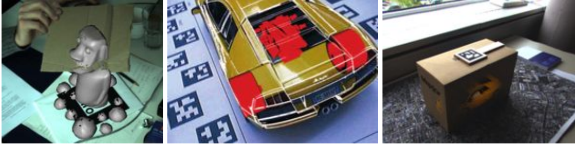
Figure 2.8: Examples for using model-based physical cues. Left) Using time-of-flight camera data for occlusion culling (Fischer et al. [34]). Middle) A ghostings based on edges extracted from a registered 3D CAD model (Kalkofen et al. [64]). Right) Using importance maps applied on a 3D model (Mendez et al. [90]).
