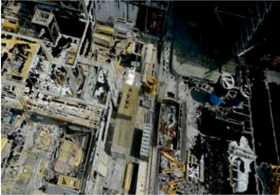
Figure 7.6: Importance driven filtering. The visibility of 3D varies based on the importance of regions in the camera image. For less important image parts, we display 3D data. In regions with important image structures, we display the camera image. This allows the user to see both, important image structures and the 3D, at the same time.
