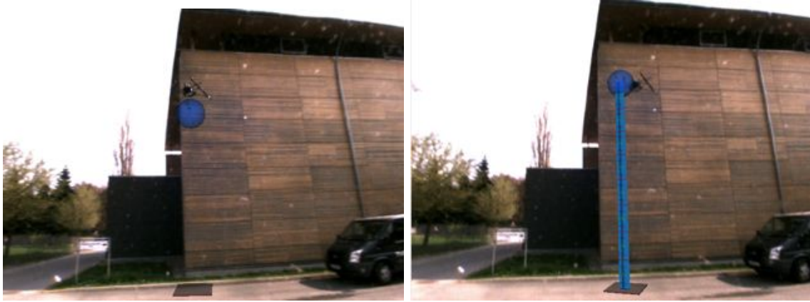
Figure 6.5: Additional graphical hints for supporting the understanding of the position of the MAV (Asctec Falcon 8 in black). Left) Sphere representation of the waypoint and its shadow projection on the ground. Right) Waypoint visualized with connection line and virtual shadows.
