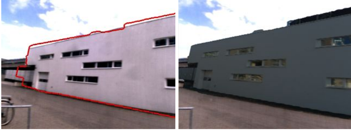
Figure 5.10: Extracted pop-up model in an AR overlay. Left) Outline of a pop-up model overlaid onto an urban scene. Right) Textured pop-up model overlaid onto the camera image.
