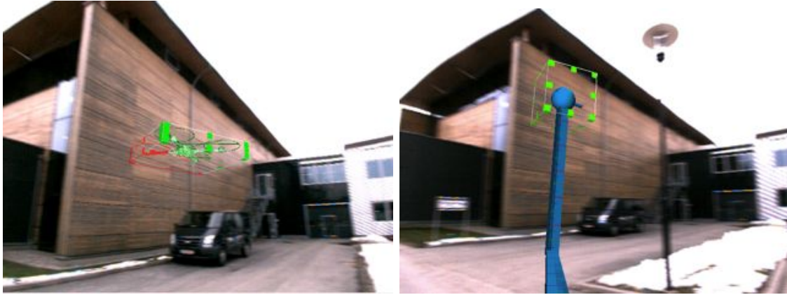
Figure 6.2: Physical cues compared to user-centric virtual cues for MAV navigation. Left) Occlusion cues for a planned waypoint of a MAV. A critical position is highlighted in red. Right) User-centric virtual cues visualize the distance between the user and the waypoint. A virtual scale texture shows the distance in meters.
