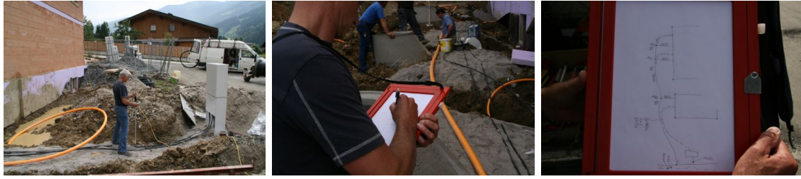
Figure 2.20: Traditional surveying methods. Left) A user surveys point of interest with the theodolite. Middle) He has to note down information about the surveyed point (such as type and id). Right) Sketching a set of surveyed points.
