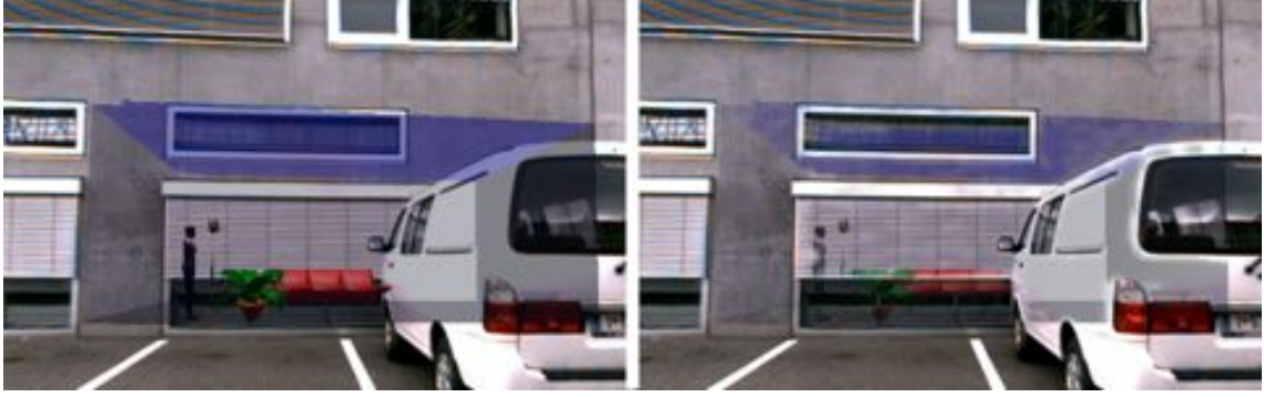
Figure 4.5: X-Ray visualization of a virtual room inside a physical building. Left) Simple overlay. The virtual room is often perceived to be located in front of the building. Right) Image-based ghostings. Occlusion cues are extracted from the video image and preserved in the visualization. The virtual room is perceived to be located inside the building.
