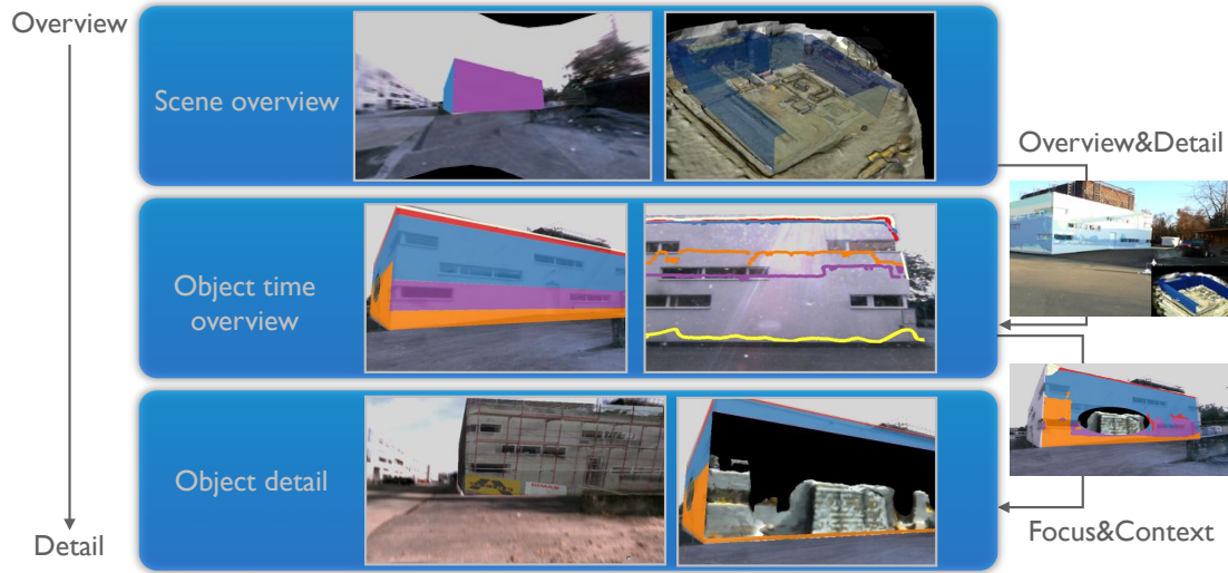
Figure 7.10: 4D visualization concept. Multiple level of detail allow to explore time-oriented data in an AR visualization. The highest level of abstraction provides just enough information to provide an overview of the data in relation to the objects in the AR environment. The second level of abstraction presents traditional time-oriented visualizations registered in AR to enable an effective analysis of time-oriented data. Its registration in AR additionally provides information about its relation to real world structure. The third level provides structural detail of the object of interest for a selected point in time and 3D space. To allow to first study the data in a higher level of abstraction before analyzing it in more detail we interactively combine all level using Overview&Detail and Focus&Context techniques.
