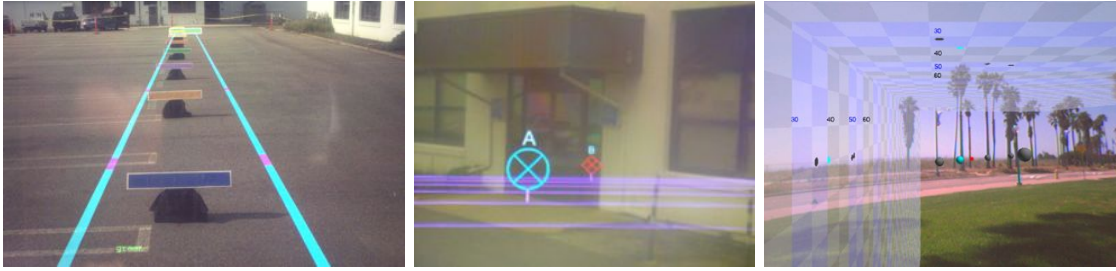
Figure 2.10: Examples for using external virtual cues. Left) Adding a set of parallel lines to improve the depth perception (Image courtesy of the U. S. Naval Research Laboratory, Livingston et al. [83]). Middle) Using a virtual ground grid to show absolute distances (Image courtesy of the U. S. Naval Research Laboratory, Livingston et al. [84]). Right) Virtual Shadow Planes for visualizing absolute depths (Wither et al. [131]).
