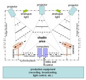
Figure 1: Modulating digital light in TV studios.
