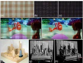
Figure 5: Projection onto a colored window curtain with and without radiometric compensation (a-e), ©IEEE. Acquired scene depth via structured light projection (f-h).
