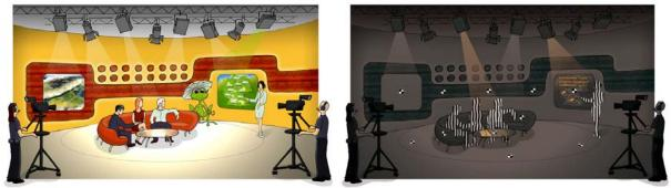
Figure 1: Digital studio illumination: Synthetic illumination studio environment with projected spatial augmentations and video augmentations (left). Embedded imperceptible patterns for scene analysis and camera tracking (right).
