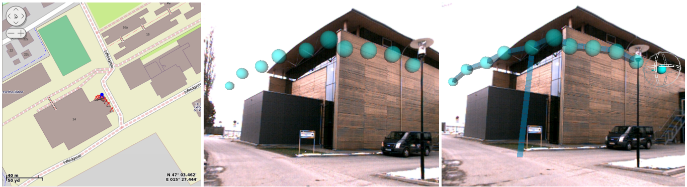
Fig. 5. Flight path visualization. (Left) Planned flight path in 2D map interface. Planned waypoints are marked with red. The current location and orientation of the aerial vehicle is marked with blue. (Middle) Planned flight path simply overlaid on imagery of the physical environment. (Right) Planned flight path visualization enriched with additional graphical hints showing the height and the distances between single waypoints. An interactive spherical modification tool allows manipulating the orientation of a waypoint.
