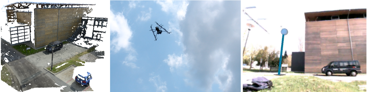
Fig. 1. Augmented Reality supported flight management for aerial reconstruction. (Left) Aerial reconstruction of a building. (Middle) The depth estimation for a hovering MAV in the distance is complicated due to missing depth cues. (Right) Augmented Reality provides additional graphical cues for understanding the position of the vehicle.
