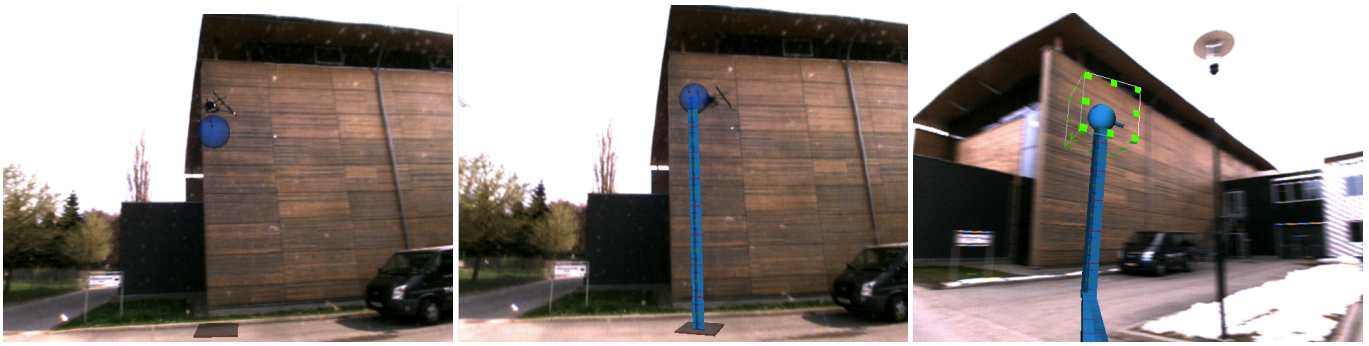
Fig. 3. Graphical hints for supporting the spatial understanding of the MAV (Asctec Falcon 8 in black). (Left) Sphere representation of the waypoint and its shadow projection on the ground. (Middle) Connection line combined with shadow. (Right) User-centric graphical cue indicating the distance of the waypoint to the user's location.
