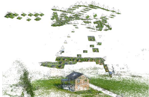
Fig. 4. Sparse point cloud and corresponding camera images.
