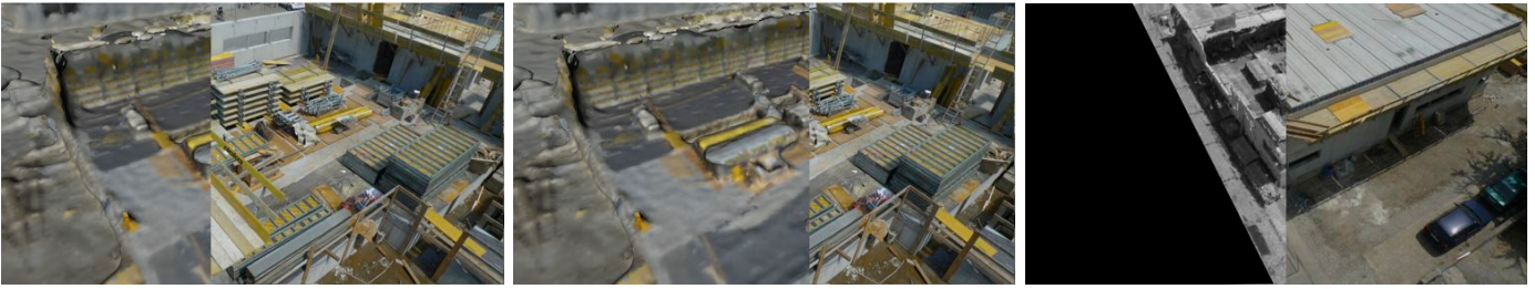
Fig. 13. Side-by-side visualization using 2D sliders. The mouse input defines the border between video image and virtual content. Left and Middle) The virtual content is overlaid on the right side of the border. Right) On the right side of the border only the virtual data representing a previous point in time is displayed.
