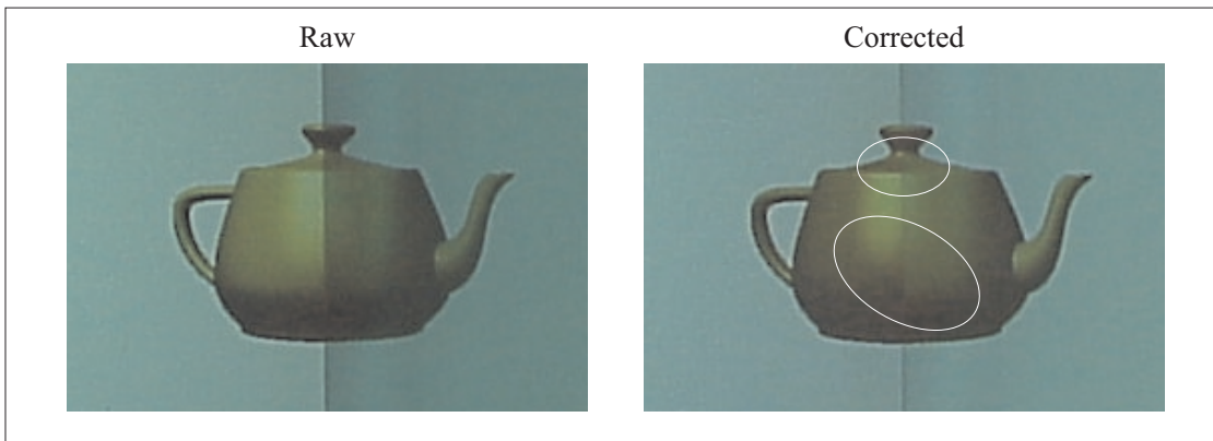
Figure 7: Imperfections in the brightness correction. A close-up of the teapot viewed at 65^\circ .
