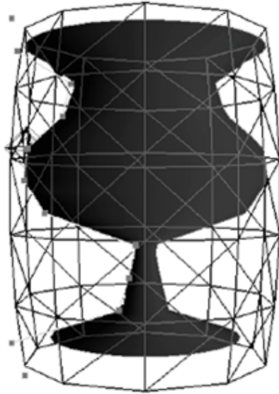
Figure 3.3: A bounding deformation mesh with control points deforming a cylinder.
