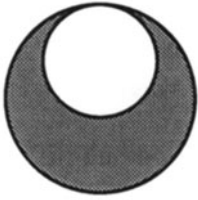
Fig. 9, Object created by subtracting spheres (in cross-section). There is a single point of no thickness at the top. This means that there is a finite hole if a very thin surface is regarded as absent.
