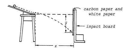
Ensure that the ramp is set so that the ball leaves it horizontally. The impact board should be firmly held to avoid movement when the ball strikes it.
