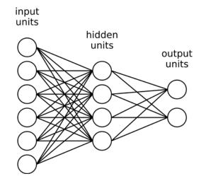
Figure 4. A simple feedforward network. (A template for a "deep network".)
